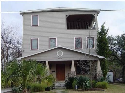
The addition is set forward flush with the front façade, but the three-story scale overwhelms the original building, and the roof form and fenestration pattern do not reflect the character of the original building.
